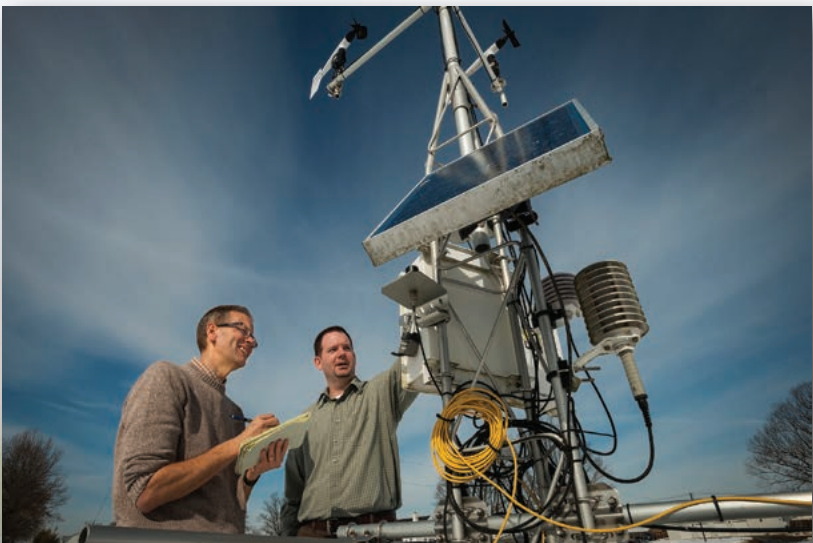
State Climatologist Dan Leathers, left, and Kevin Brinson inspect a Delaware Environmental Observing System (DEOS) weather station.
